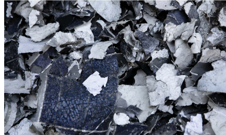
Figure 11: Crushed PV panel materials. Sourced from "Scoping Study: Solar Panel End-of-Life Management in Australia", ACAP, March 2024
