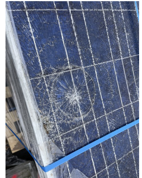
Figure 8: A broken solar panel at a PV recycling facility
