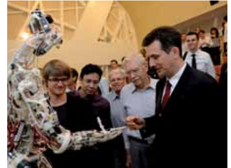
The Eccerobot, a soft robotics approach to understand human intelligence from the Artificial Intelligence Laboratory of the University of Zurich (in Singapore in April 2011)
