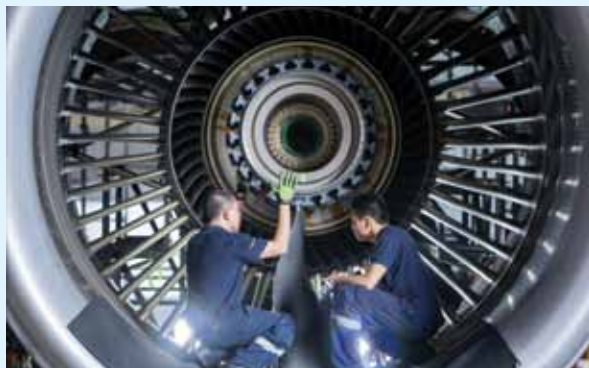
LTP mechanics reattaching the engine blades of an Airbus A380, the biggest passenger aircraft in the market today
