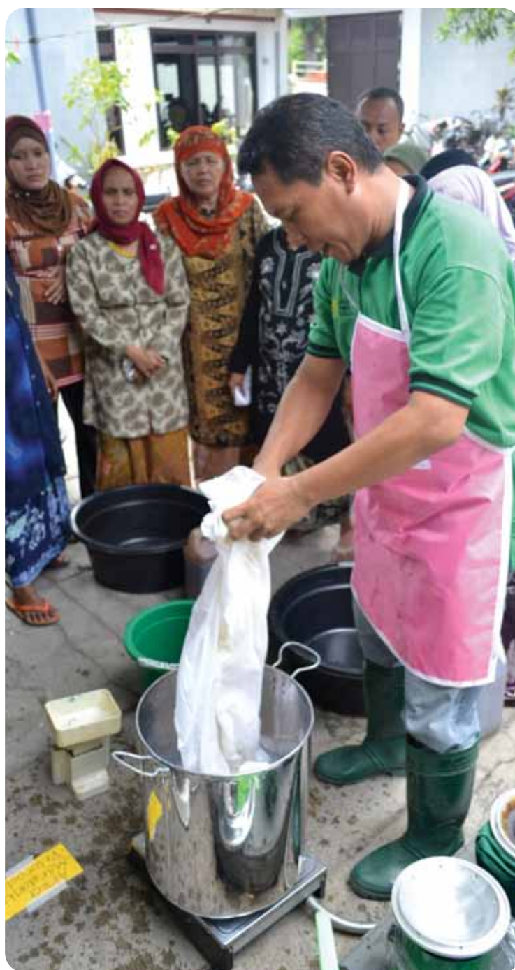
Clean batik. Melting the wax used in batik with electric instead of kerosene stoves greatly reduces energy costs and workplace pollution.
