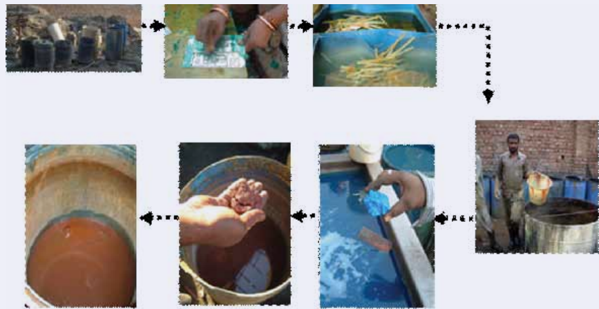
Figure 7 Acid Bath Process
