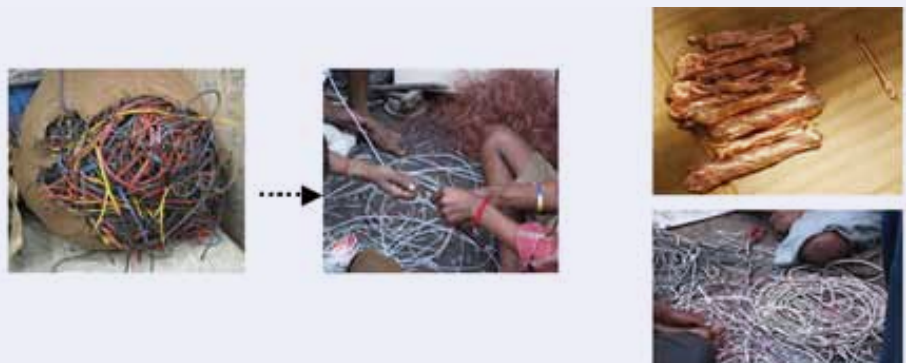
Figure 4 Extraction of copper from wires through manual drawing
