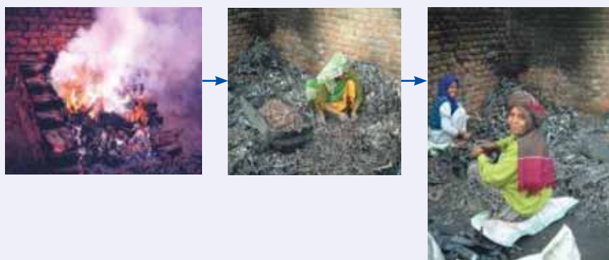
Figure 6 Open burning of PWB for copper extraction
